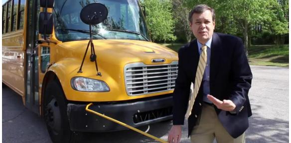
In the new boarding process, students will wait until the crossing control arm fully deploys before leaving their bus stop to board the bus.
